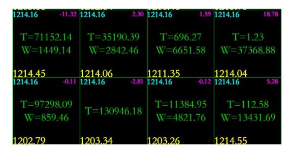
In the figure, T represents the amount of filling and W represents the amount of digging. The yellow number near each grid node represents the elevation of the corresponding point cloud of the grid dot, the blue number represents the elevation of the reference surface, and the pink number represents the difference between the two.
